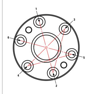
It is recommended to tighten the bolts equally by diagonal sequence as indicated in the drawing;
