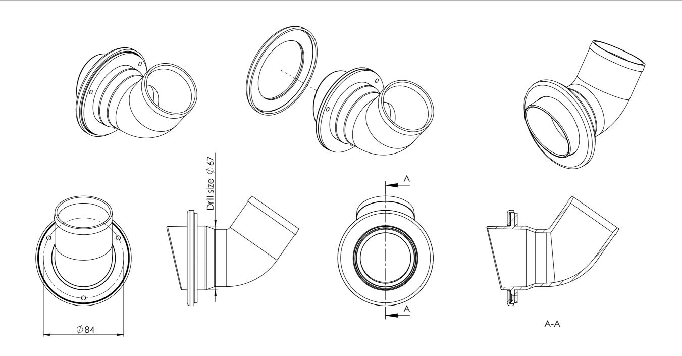
Maximum hull thickness: 26mm Drill size: ø67mm PCD: ø84mm, countersunk ø4.2mm
